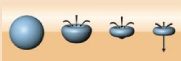
Schematic drawing illustrating the development of a microjet.
