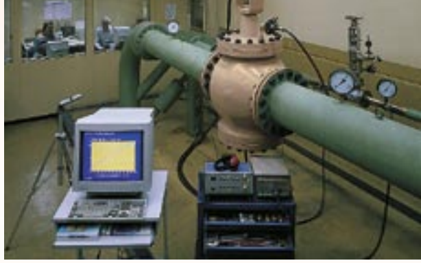
The valve-specific x_{Fz} values are determined on test rigs, enabling the prediction of the noise level and erosion behavior.
