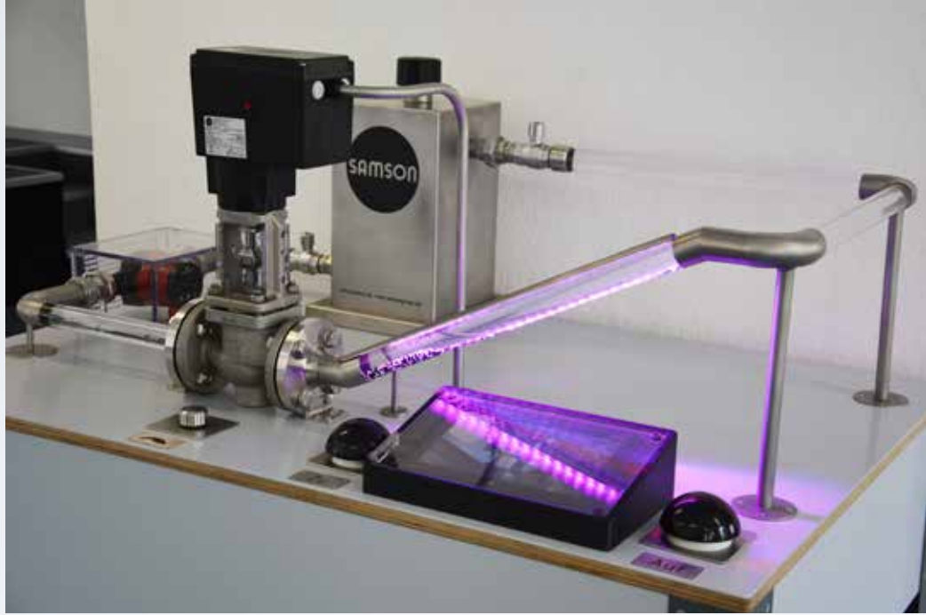
Visitors of the EXPERIMINTA museum can directly change the valve position in the exhibit, which simulates flow control, using potentiometers.
