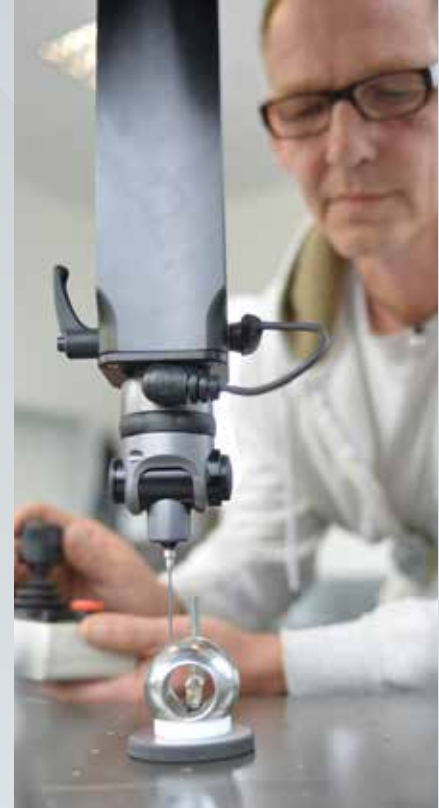
Every incoming component is subjected to 3-D measurements and other material quality inspections.
