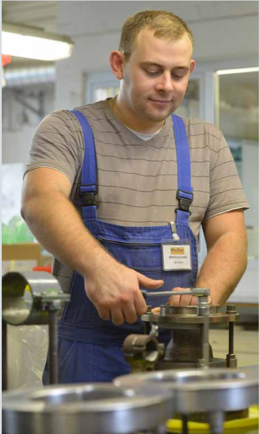
The PTFE-lined ball valve is prepared for hot isostatic pressing where the powder is turned into a compact plastic.
