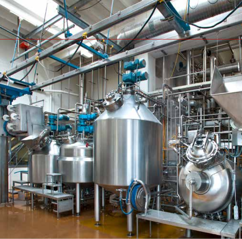
Typical control tasks performed by the electric actuator with process controller include controlling the temperature in pasteurization processes in dairies. The milk is briefly heated up to extend its shelf life.
