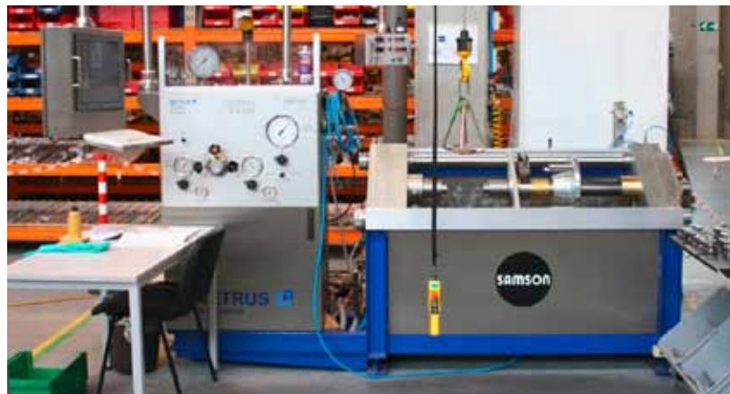
At Antwerp, complete control valves can be assembled and tested.
