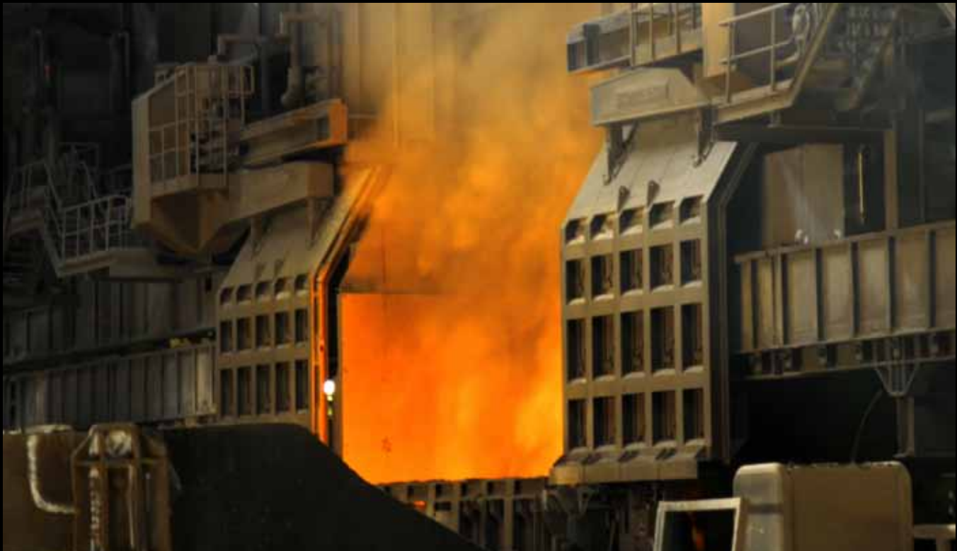
The iron ores are reduced in a blast furnace. The carbon-rich molten raw iron is converted into low-carbon steel in massive converter ladles
