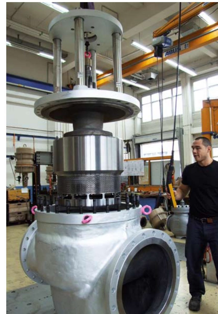
...to final assembly: manufacture of the blow-off valves specifically designed to protect the axial flow compressors in the Indian steel plant at Rourkela was entirely performed by SAMSON.
