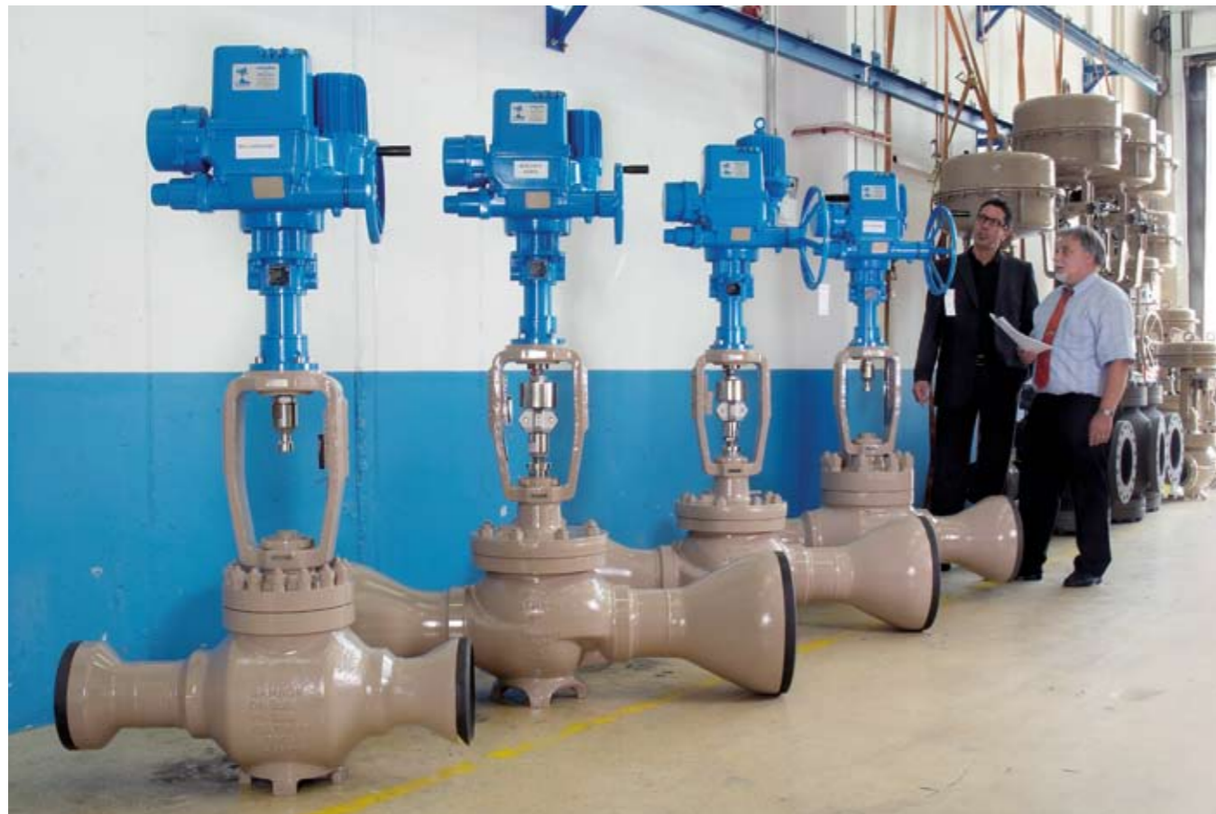
Some of the control valves for the new coal-fired power plant at Wilhelmshaven are ready for the final acceptance test by the customer.
